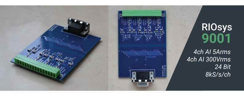
The RIOsys 9001 is a differential analog input for 4 voltage and 4 current channels. The wide measurement range is well suited for high-voltage and current measurement applications such as power metering, power quality monitoring, etc.
